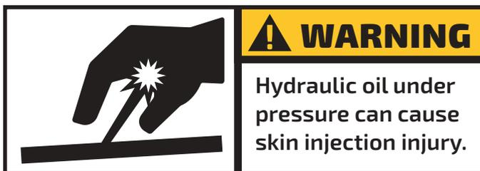
To lessen the potential of injury due to stored energy, lower the ripper to the resting position and relieve all hydraulic pressure before performing maintenance.
