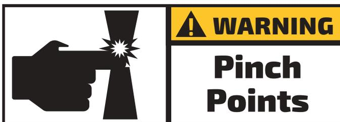
This attachment contains areas that have the potential to pinch, snag, or crush. During operation, keep a safe distance from moving parts and avoid wearing loose fitting clothing and jewelry.
