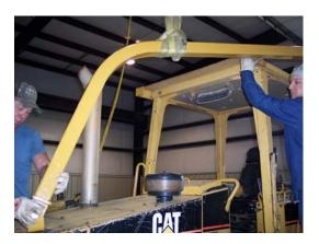
5. The front soft mount swivel does not have the weld plate welded on it. Once the front end of the sweep arm is trimmed you then should tack weld the loose weld plate to the arm. See picture below.
