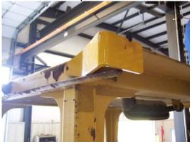
3. The front soft mount swivel has been sent with the sweep arm weld pad loose. Place these soft mount swivels on the hard nose brackets allowing the stobs to be parallel with each other. This will allow the sweeps to be unbolted from the cab and swivel over the blade for future maintenance. See the picture below!
