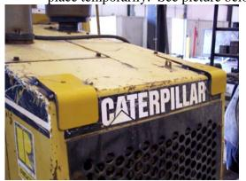
2. The cab brackets go on the side and the front of the cab to allow a flat area for the sweeps to weld to. You will need to grind the areas that will be welded before the brackets are tack welded to the cab. The brackets fit on the cab as shown in the picture below!
