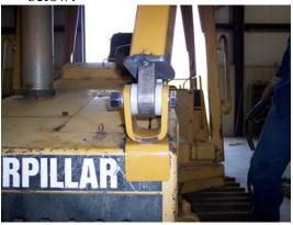
4. Using a lifting device such as a forklift or an overhead crane, lift one of the sweep arms up on the machine and simulate how the arm will be mounted to the machine. Take the soft mount swivels and hold them in place to mark where the arms are to be trimmed. The arms are sent long to give extra for different mounting styles. See picture below!
