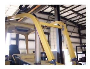
8. Weld all welds with at least a 1/4" fillet weld.
