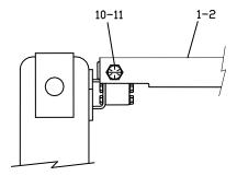
Step 4 Go back to the hardnose end of the sweep group and fit the 2 rubber bushings (9S5187D) into the stobs of the sweep group and then bolt the U- brackets to the stobs using the 2 bolts (1" X 4-1/2" NC) and 2 lockunts (1" NC). The bolts should not be tightened at this time. The U-brackets should be sitting on the hardnose plates as indicated in the view below.
