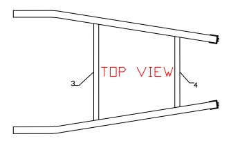
Step 6 Now that everything is basically in place, you should go back and tighten all bolts and weld out the hardnose plates, U- brackets & cross tubes. All welds should be minimum 1/4" fillet weld.
