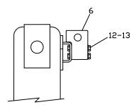
Step 2 Place the hardnose plates (SP0008) on the hardnose, spacing them 14-1/2" off the center of the hardnose as indicated the drawing below. Tack weld the plates to the hardnose.
