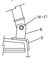
Step 5 Now tack weld U-Brackets to Hardnose and tack weld cross tubes in their appropriate places as seen in view below.
