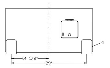
Step 3 Place the RH & LH sweep arms (SP0045 & SP0046) in place on the machine. The sweep arms have been notched out to fit over the mounting blocks. The sweep arms need to be placed on top of the mounting blocks. This will be a tight fit. Align the holes in the sweep group and the mounting blocks and use the 2 bolts (1" X 5" NC) and the 2 locknuts (1" NC) to secure them together. The bolts should not be tightened at this time.
