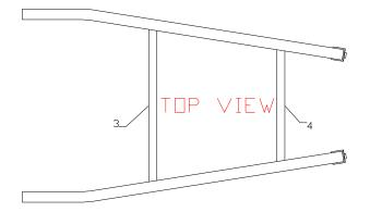
Step 6 Now that everything is basically in place, you should go back and tighten all bolts and weld out the hardnose plates, U- brackets & cross tubes. All welds should be minimum <sup>1</sup>/<sub>4</sub>" fillet weld.
