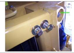
**\*\*NOTE**\*\*At this point, the side (2) bolts do not need to be loosened, as shown above. They are for adjustment only as needed.
