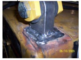
\*The sweeps should be checked to make certain that they do not interfere with any operation of doors before solid welding.
