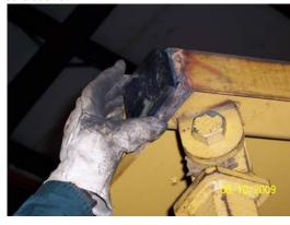
Weld the hardnose bracket to the corners of the nose of the tractor.
