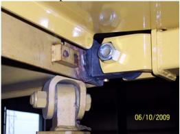
Allow the front weld stobs to come down into contact with the hardnose mounting plates on the nose of the tractor, and tack weld in place.
