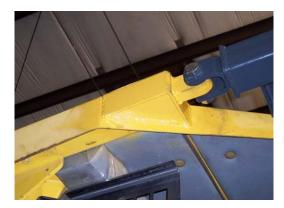
• Lift Sweep Body into place allowing weld stobs to center on the Cab Brackets.
