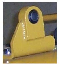
Lift the SP0135 Sweep Body with a hoist or overhead lift over the tractor & align with all 4 brackets and bolt to Cab Brackets and Hard Nose Brackets using 1-1/2" Wrench (1), 1" x 4-1/2" Bolts (4), 2" Lock Nuts (4), 9S5187D Rubber Mounts (4) & 8P5244D Rubber Washers (8). See 2 Pictures below...
