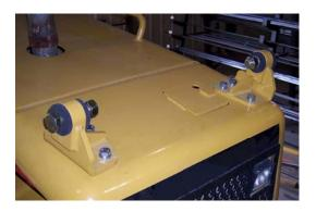
• Insert 9S5187D Rubber Mounts (4) into Cab Brackets & Hard Nose Brackets using a rubber mallet as seen below...
