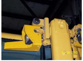
\*Note optional Light & Light bracket has been bolted to Cab Brackets above which can be done using 9/16" Wrench (1), 3/8" x 1" Bolts (8) & 3/8" Lock Washers (8) supplied.
